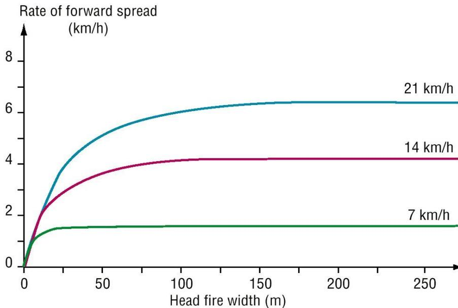
**Figure 6. Relationship describing the rate of spread that will be attained by grassfires burning at different head fire widths at increasing wind speeds.**
