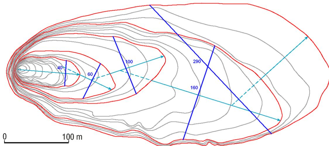
**Figure 1. The progress of an experimental fire, ignited at a point. The red perimeters show the size of the fire at the time the wind direction changed; the light blue lines show the direction of the wind and the axis along which head-fire spread was measured.**
