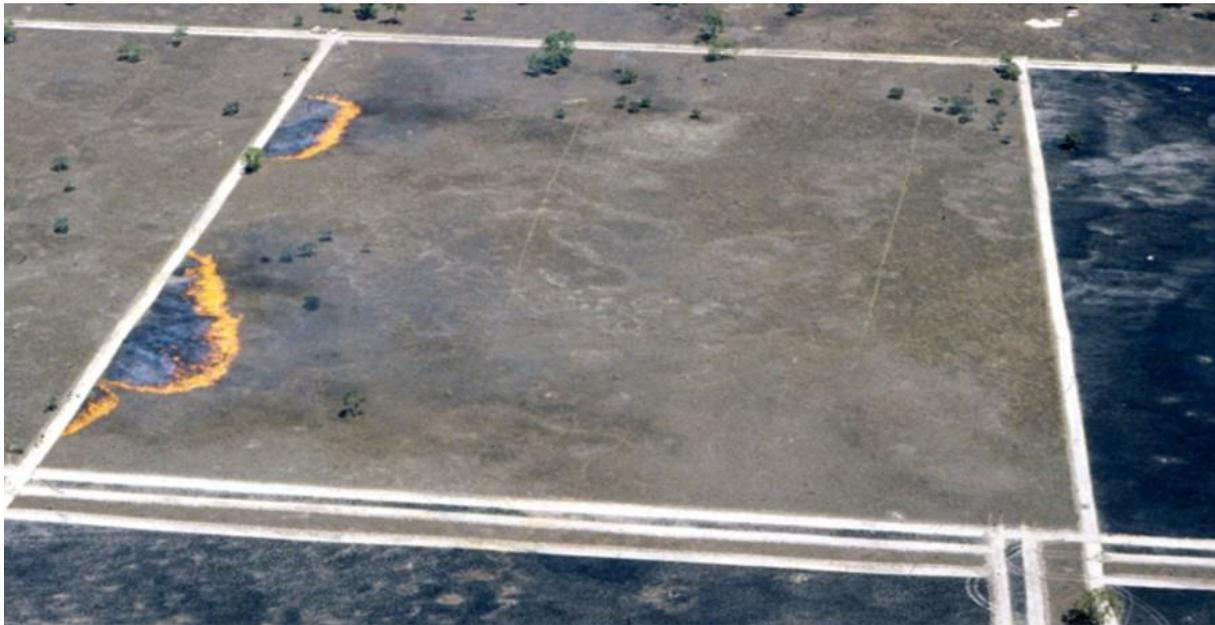
**Figure 3. Grass fires lit at a point, 50 m line and 100 m line after 40 seconds. The 100 m line is not yet complete. The point ignition is barely visible at the top centre of the plot. (need to insert arrows)**
