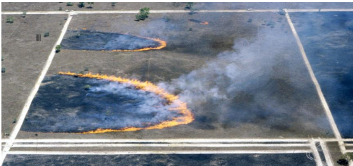
Figure 4: Simultaneously lit grass fires 100 seconds after ignition.
