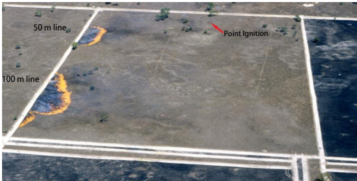
Figure 3. Grass fires lit at a point, 50 m line and 100 m line after 40 seconds. The ignition of the 100 m line is not yet complete. The point ignition is barely visible at the top centre of the plot.
