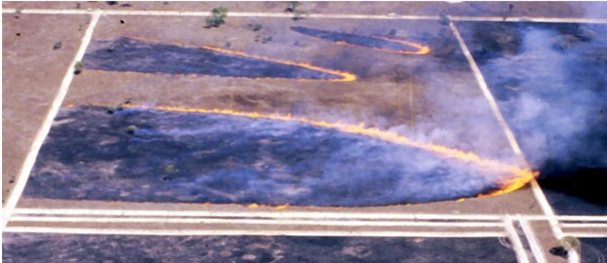
Figure 5: Simultaneously lit grass fires 160 seconds after ignition
